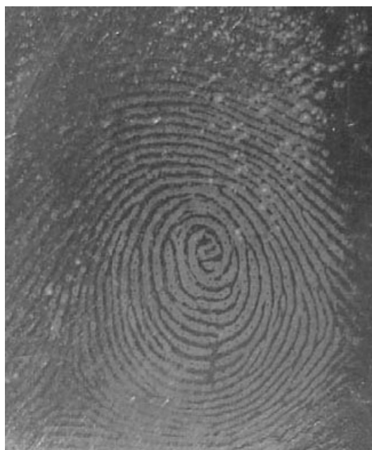
FIG. 9—Fingerprint corrosion on brass disk (disk C) that gave no coherent \Delta V and did not exhibit the characteristics of a Schottky barrier.
